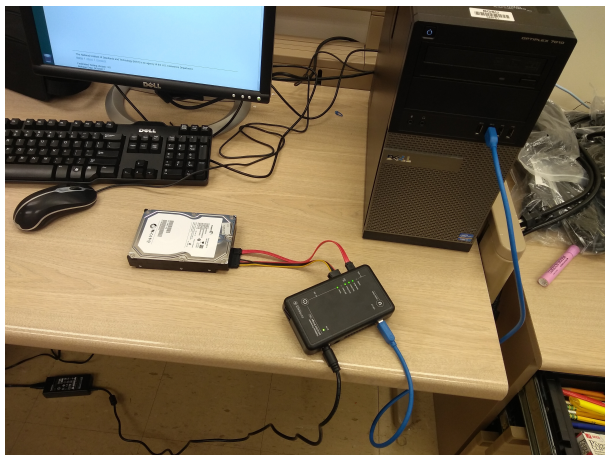
Fig. 1. The lab setup: The HWB device (which is under evaluation) is placed in the middle of the hard disk (which is under protection) and the host computer (running NIST CFTT Federated Testing System).
